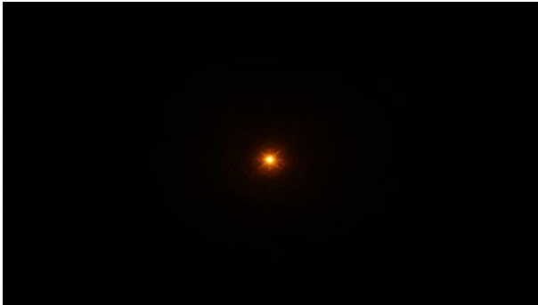
Point spread function for optical test set-up without test object
